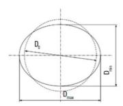
D0 is the arithmetic mean between the smallest and biggest tube diameter on any one pipes or tube circumference. If minimum wall thickness is required variations are allowed on the plus side only
